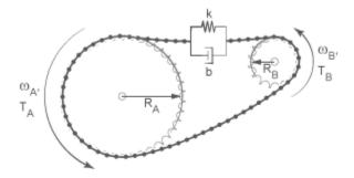
The chain tensile force is the net sum of spring and damper forces. The spring force is the product of the tensile strain and the spring stiffness constant. This force is zero whenever the tensile strain is smaller than the chain slack. The damper force is the product of the tensile strain rate and the damping coefficient. Mathematically,
