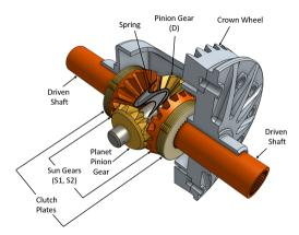
The Limited-Slip Differential block models the LSD mechanism as a structural component based on the Simscape Driveline Differential and Disk Friction Clutch blocks. The differential mechanism modeled by the Differential block is a structural component based on two other Simscape Driveline blocks, the Simple Gear and the Sun-Planet Bevel. The block diagram shows the structural components of the LSD.
