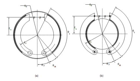
In this schematic, a) represents an internal double-shoe brake, and b) represents an external double-shoe brake. In both configurations, a positive actuation force F brings the shoe and drum friction surfaces into contact. The result is a friction torque that causes deceleration of the rotating drum. Zero and negative forces do not bring the shoe and drum friction surfaces into contact and produce zero braking torque.
