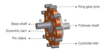
During normal operation, the base shaft drives the eccentric cam. The cam spins inside the cycloidal disk, causing it to rotate in an eccentric pattern about an offset axis. As it moves, the cycloidal disk engages the internal teeth of the ring-gear housing. The internal meshing reverses the rotational velocity direction.
