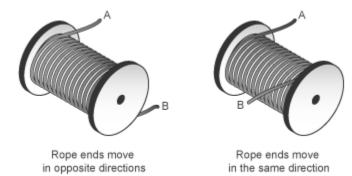
During normal operation, a driving torque causes the cylindrical drum to rotate about its symmetry axis. The rotating drum transmits a tensile force to the rope ends, which translate with respect to the drum centerline. The relative direction of translation between the two rope ends depends on the rope windup type. However, a positive drum rotation always corresponds to a positive translation at rope end A.
