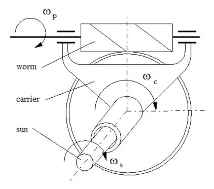
You specify a fixed gear ratio, which is determined as the ratio of the worm angular velocity to the sun gear angular velocity. You control the direction by setting the worm thread type, left-handed or right-handed. Rotation of the right-handed worm in positive direction causes the sun gear to rotate in positive direction too. The positive directions of the sun gear and the carrier are the same.
