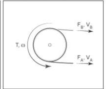
The translational velocities of the two rope ends are functions of the drum radius and angular velocity. Each translational velocity is equal to the tangential velocity of a point at the drum periphery according to the expressions:
