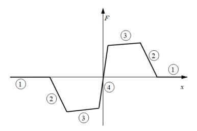
Because the ball is spherical and the notch is symmetric, the horizontal force versus displacement function is symmetric about the origin. (See "Peak Force and Notch Width" on page 1-431.)
