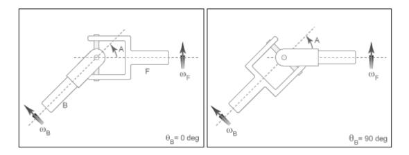
In the figure, the intersection angle is the angle between the two shafts about the pin of the base shaft. The absolute value of this angle must fall in the range 0≤A<Maximum intersection angle. The base shaft angle is the angle of the base shaft about its
